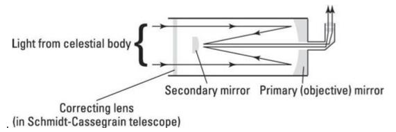
Because of their design, Cassegrain reflectors can be more compact than their Newtonian cousins, because the light is 'folded' twice inside the tube, making two journeys rather than one. Cassegrain telescopes can be half the length of Newtonians. Cassegrain reflecting telescopes have all the same advantages as a Newtonian reflector, plus they're much more compact
