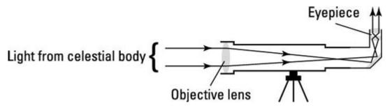
This setup can make observing through a refracting telescope quite uncomfortable, especially if you're pointing your telescope high in the sky, because you may have to stoop and crane your neck to see through the eyepiece. Some telescopes come with a prism adaptor that bends the light through 90 degrees, so looking through the eyepiece is much more comfortable.
